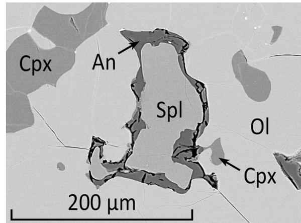
Fig. 1. Backscattered electron (BSE) image of NWA 14758, showing the reaction at the edges of spinel to form anorthite. Spl = spinel, An = anorthite, Ol = olivine, Cpx = clinopyroxene.
