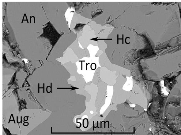
Fig. 3. The BSE image of a late-stage assemblage in NWA 15507. Tro = troilite, Hc = hercynite, Hd = hedenbergite, An = anorthite, Aug = augite.
